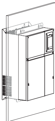
Figure 3-11 Embedded installation effect of the VDF650 (sheet metal housing)
