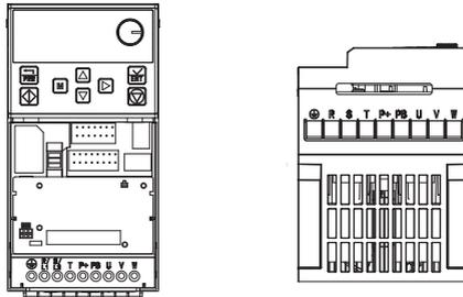
Figure 3-9 Terminal arrangement in VDF750T0.7GB to VDF750T55G
