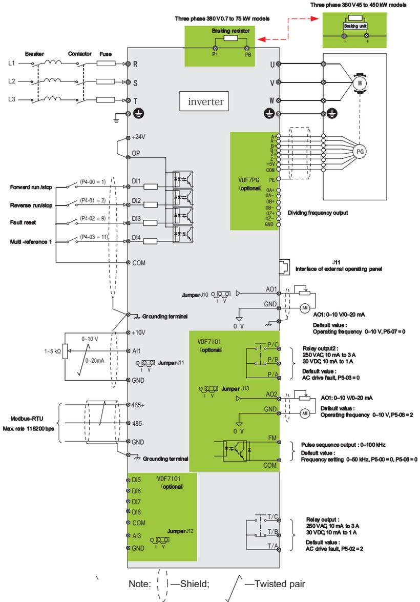
Figure 3-8 Typical wiring
