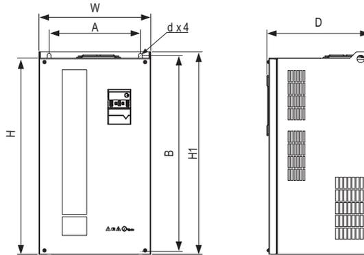
Figure 1-6 Overall and mounting dimensions of VDF750T30G(B) to VDF750T185G and VDF750-2T15GB to VDF750-2T55G
