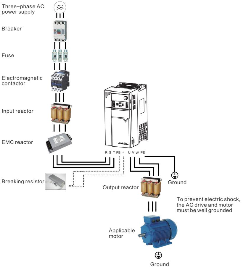
Figure 2-1 VDF750 series system composition
