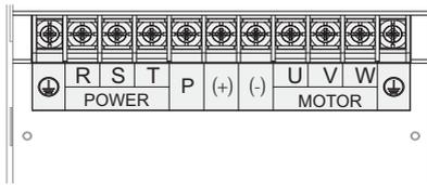
Figure 3-10 Terminal arrangement in VDF750T75G to VDF750T185G
