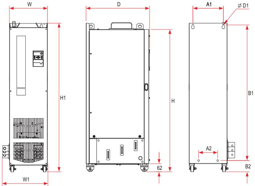
Figure 1-7 Overall and mounting dimensions of VDF750T200G to VDF750T450G
